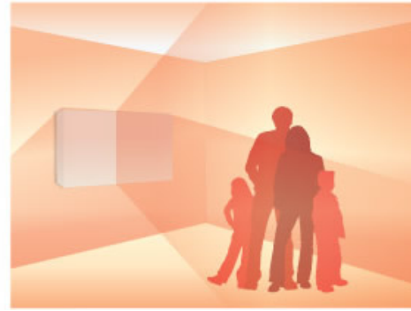
LAVA Infrared Radiant Heating works by evenly warming the fabric of the room which in return radiates heat efficiently
